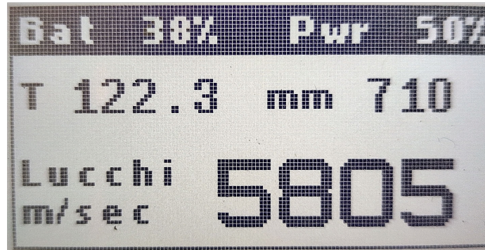
Figure 3.2 — LucchiMeter PRO LCD display during a measurement, showing Bat, Pwr, mm and Lucchi value in m/sec
