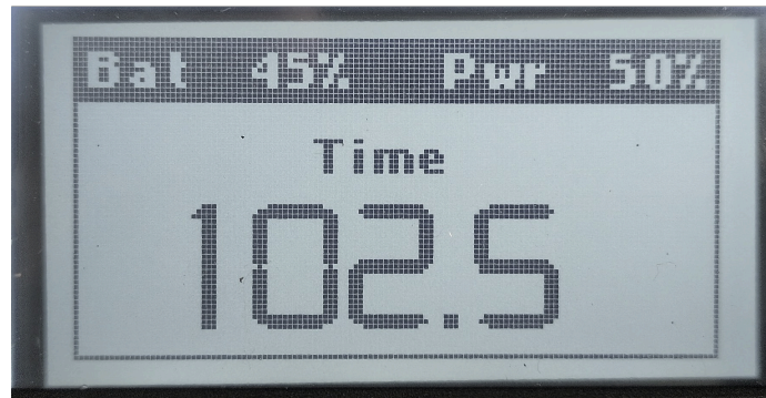
Figure 3.2 — LCD display of the LucchiMeter BASIC during a measurement, showing Bat, Pwr and Time in microseconds
