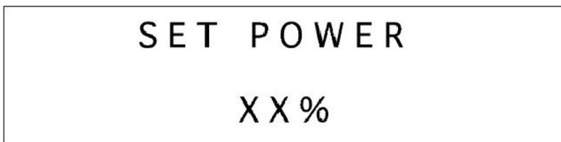
Ultrasound pulse power can now be varied using the UP and DOWN keys.
