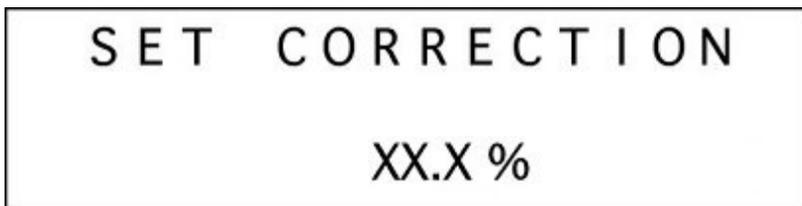
The UP and DOWN keys will allow to set the correction coefficient needed to correct particular characteristics of the measured sample (humidity, shape, presence of foreign inclusions into the material). To return to measurement mode, push the LUCCHI key or wait 5".
