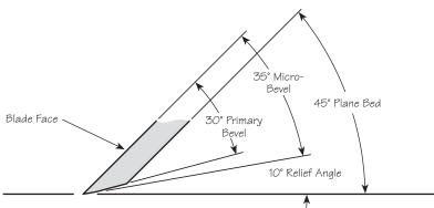
Figure 4: Blade with micro-bevel.
