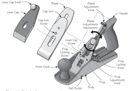
Figure 1: Bench plane components.
