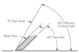
Figure 5: Blade with back bevel.
