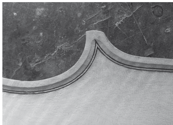
Fig. 13 - ...quindi terminava la sguscia / ...and completed the channel
